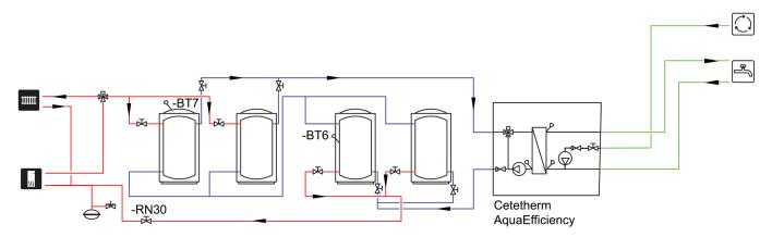
Note! The flow in the blue pipes are higher than in the red pipes.
